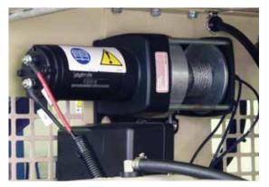
Single internal electrical winch "one man easy operation".
